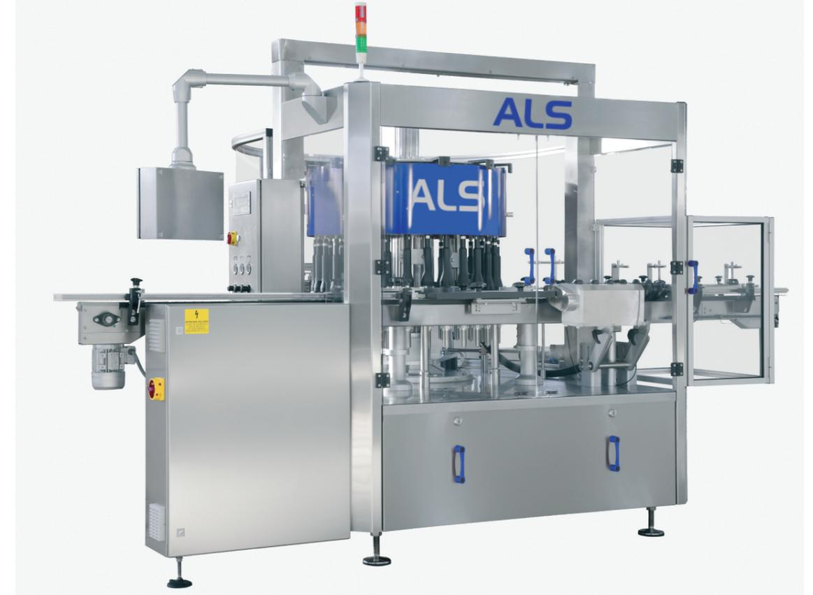
High-speed, high-volume application of front/back, multi-sided, neck, recessed & wrap-around labels.
